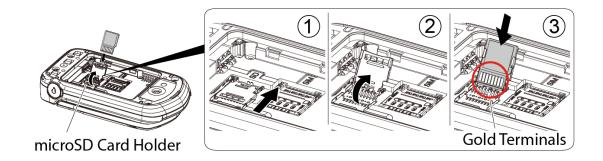
4. Gently press the card and the card holder (4), and then slide the holder in the direction of the arrow to lock it (5).
