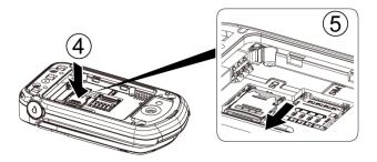
5. Place the battery back into its compartment and replace the battery cover. See Install the Battery.
