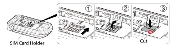
5. Replace the SIM card holder (4) and slide the holder in the direction of the arrow to lock it (5).
