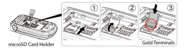
5. Gently press the card and the card holder (4), and then slide the holder in the direction of the arrow to lock it (5).
