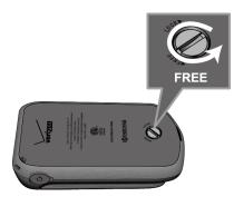
**Note:** The battery cover screw is permanently mounted on the cover and cannot be removed.
