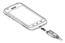
• Plug the other end of the USB cable into the charger, and then plug the charger into an electrical outlet.
