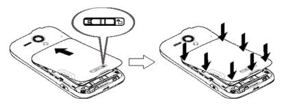
• Slide the battery cover lock to the locked position.
