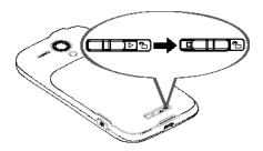
• Insert your thumbnail or fingernail into the slot and lift the battery cover gently.
