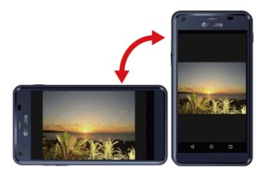
**Note**: The Auto-rotate feature needs to be turned on for the screen orientation to automatically change. From home, tap **Apps Settings** > **Accessibility** > **Auto-rotate screen**.
