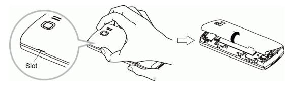
• Insert the battery, contacts end first, and gently press the battery into place.
