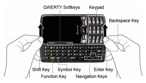
**Note:** When the slide-out keyboard is opened, the display stays in landscape mode and you can use the keypad on the front panel for entering numbers.
